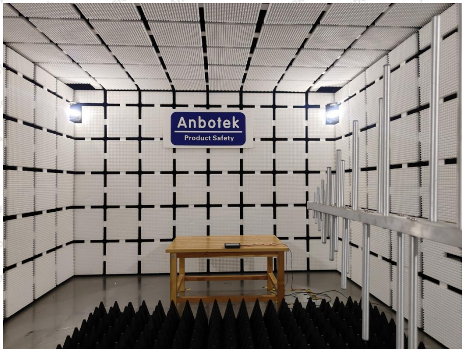
Photo of RF Field Strength Immunity Test
