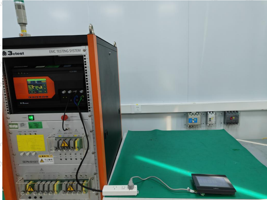
Photo of Electrical Fast Transient/Burst Immunity Test
