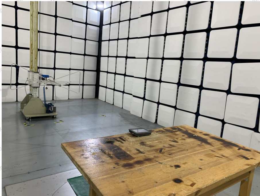
Photo of Radiated Emission Test (Below 1 GHz)
